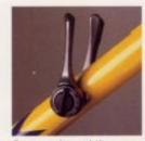
Suntour Accushift indexing gives you precise control of 12-speed gearing with just the flick of a finger.
